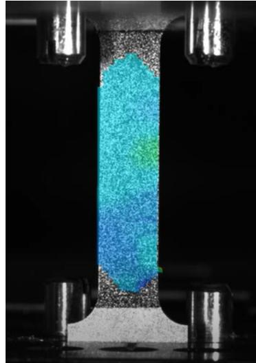
(b) Major strain of tensile test sample 6.1 before it starts to neck.
