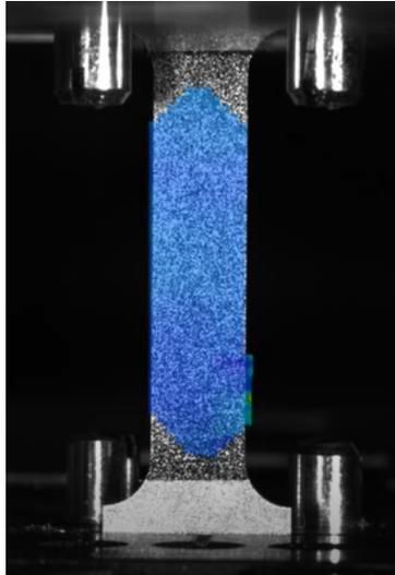
(a) Major strain of tensile test sample 6.1 halfway until it starts to neck.
