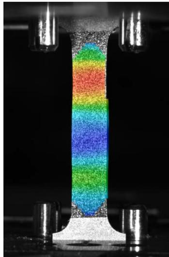
(b) Major strain of tensile test sample 2.2 before it starts to neck.
