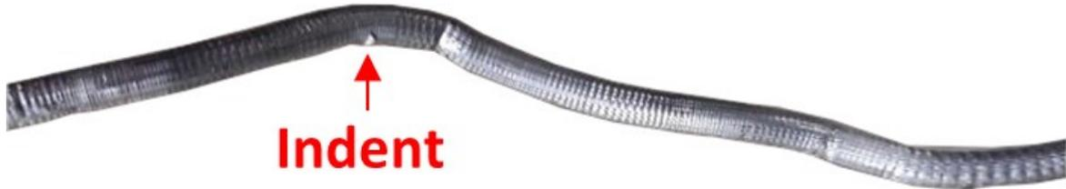
**Figure B.4:** Example of an extruded specimen.
