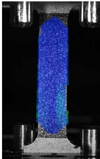
(a) Major strain of tensile test sample 7.2 halfway until it starts to neck.
