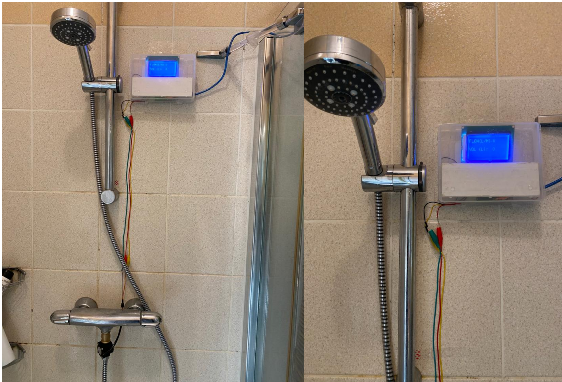
Figure 9: Shower setup with screen and flowrate sensor
