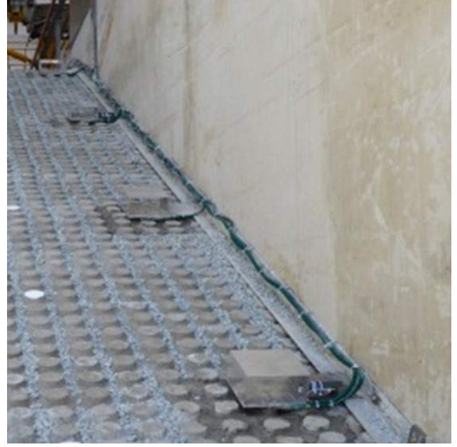
(b) Pressure sensors 2 - 5 located on inner slope.
