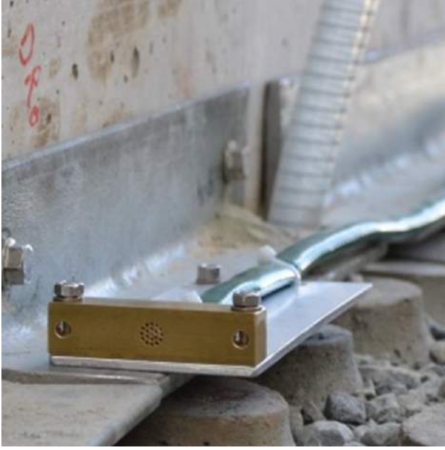
(a) Pressure sensor 1 located on the crest.
