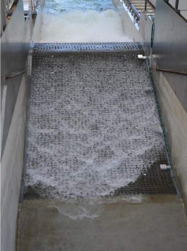
(a) Wave overtopping during the test.
