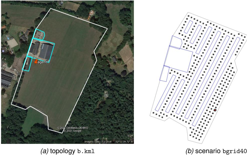
**Figure 5.2:** Google Earth topology and resulting simulation environment. The landmarks (grey dots) are based on a grid. The agent origin (red dot) is randomly relocated. Row obstacles are added to simulate rows of crops.
