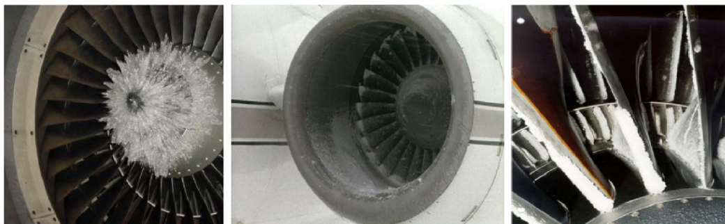
Figure 1.1: Examples of ice accretion due to supercooled droplets on different parts of a turbofan engine. From left to right ice accretion is shown on the spinner of the fan, near the tip of the fan blades and near the base of the fan blades on the pressure side in a close up view [2].
