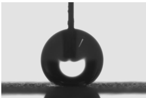
Figure 10: Image from the Dataphysics OCA. Shown is a water droplet of about  $4\mu\text{l}$  with the syringe used for deposition still sticking in it.
