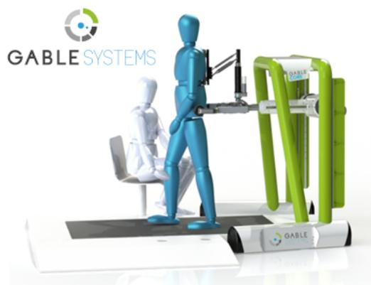
Figure 1.1: Gable Core gait and balance training platform: bodyweight is compensated at the hip. The mobile base and internal actuation facilitate impedance reduction, such that the robot follows the freely moving user unobstructed. Supportive or resistive forces can be applied for training purposes.
