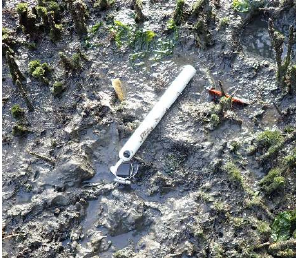
Figure 2.5: Lowell TCM-4 Tilt current meter. Photographed by Erik Horstman.
