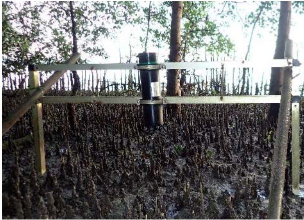
Figure 2.7: Echologger EA400 placed in frame. Photographed by Erik Horstman.
