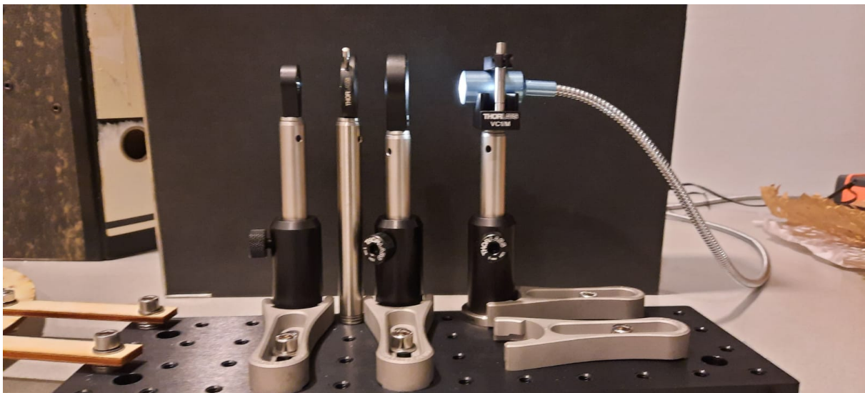
Figure 10: A picture of the set-up that is used to collimate the white light fibre source.
