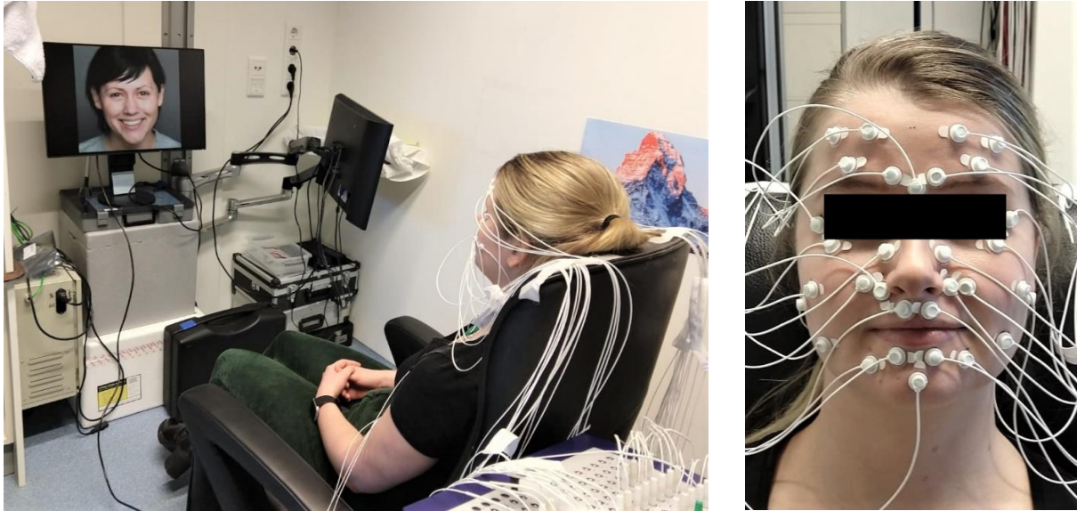
Figure 14: Pictures taken during the experiment. The subject is seated in a chair in front of a screen on which stimuli are presented (left), the used electrode configuration (right).
