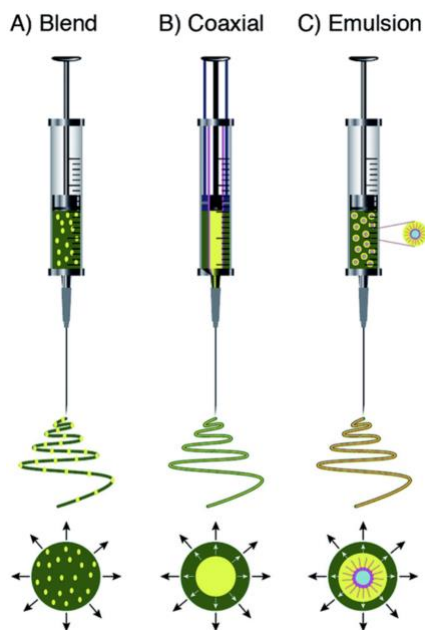
Figure 9 : The difference in the loading of the polymer-solvent solution (dark green) with the therapeutic agent (light green) for blend, coaxial, and emulsion electrospinning and the difference in the resulting structure of the nanofibers [43].
