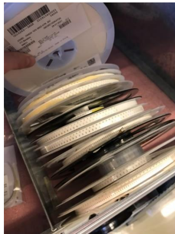
Figure 2.3. Components on a reel in GE's warehouse.
