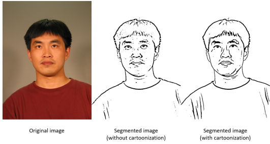
Figure 4: Output of adaptive thresholding segmentation for an image with and without cartoonization.
