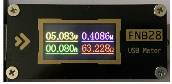
Figure 2. FNB28 USB Power Meter Interface
