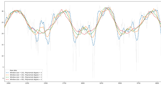
Figure 6. Comparison of Savitzky Golay filters with different window lengths, polynomial degree = 3
