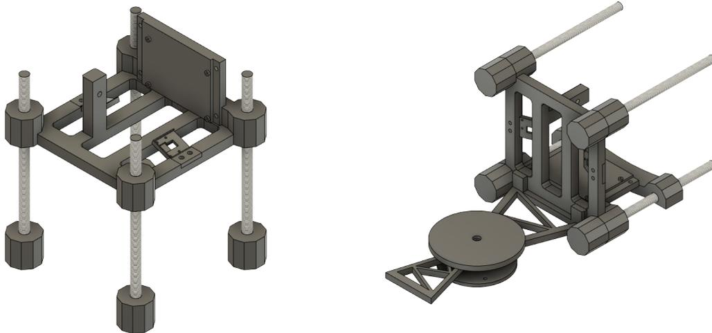
Figure 10: 3D designs of the prototype handheld scanner and the rotary test platform
