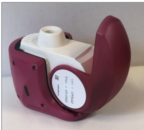
Figure 2: The AMIKO Respiro™ add-on device connected to the NEXThaler inhalator.
