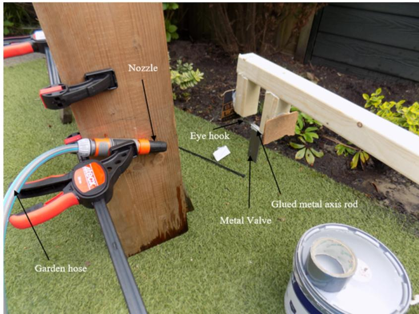
Figure 9: Impression of the physical experimental setup used to test the gravity driven pivot valve theory.
