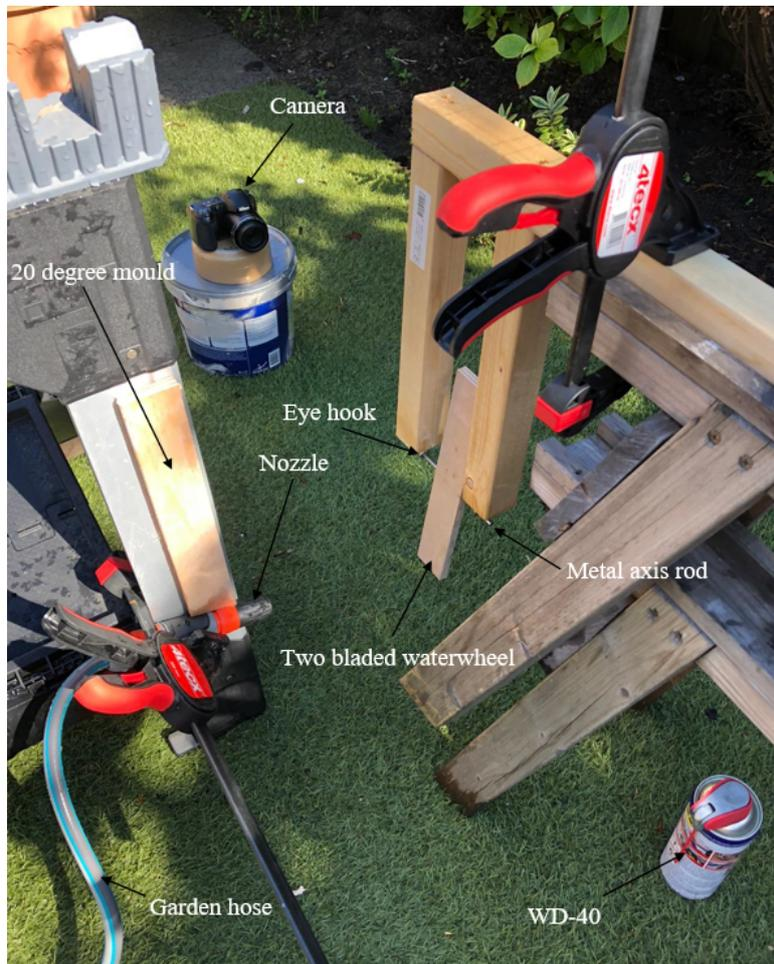
Figure 10: Impression of the physical experimental setup used to test the waterwheel theory.
