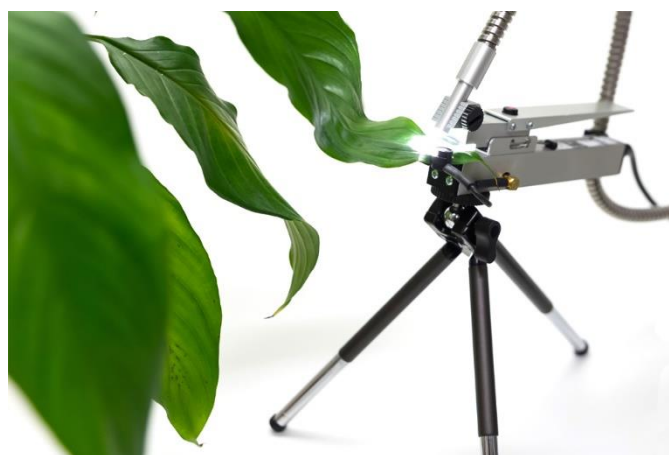
Figure 13: FMS/PTL leaf clip from Hansatech instruments
