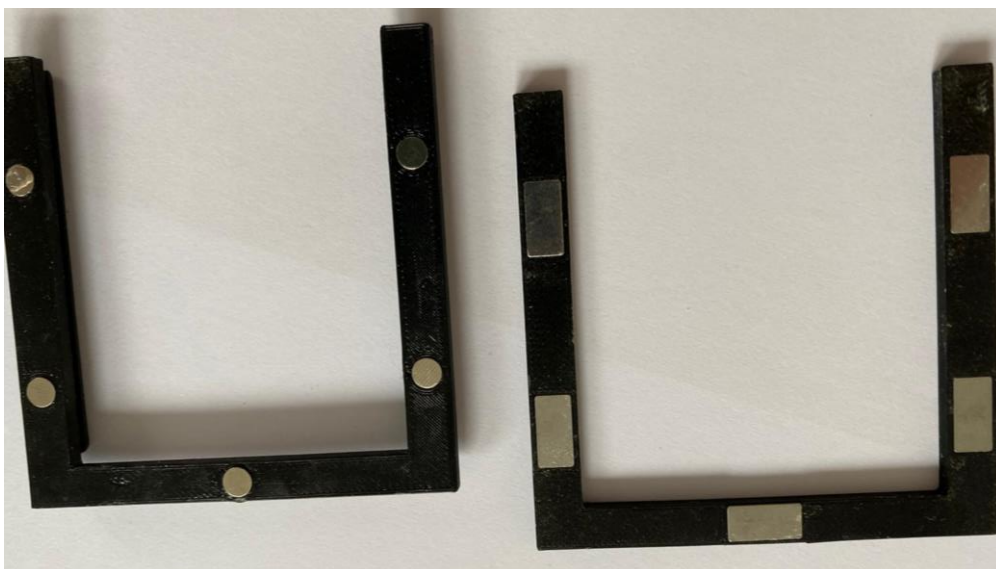
Figure 29: magnets and metal plates glued onto the leaf clip
