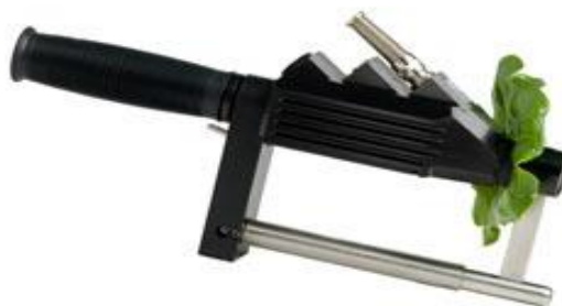
Figure 11: ASD spectrometer plant probe
