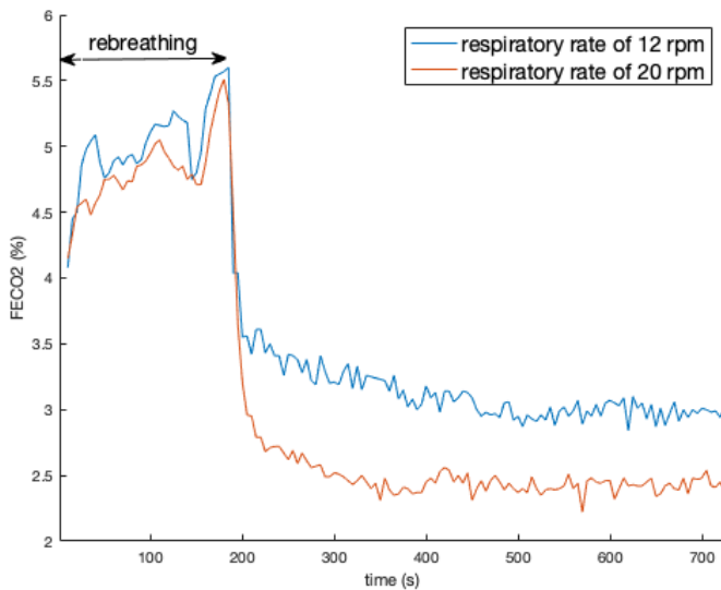
Figure 16 The averaged graphs belonging to measurement 2 and 3. The transient response of the fraction of the expired \text{CO}_2 after a period of rebreathing is displayed.
