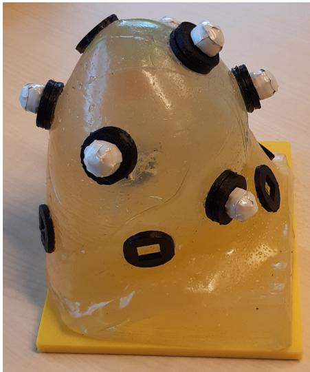
(a) The phantom with relevant markers attached
