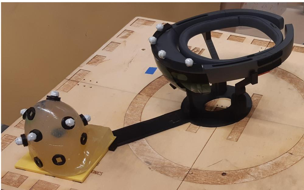
Figure 15: HoloLens stand connected to the phantom. The stand can be attached to any of the 4 corners of the orange plate on which the phantom is placed.
