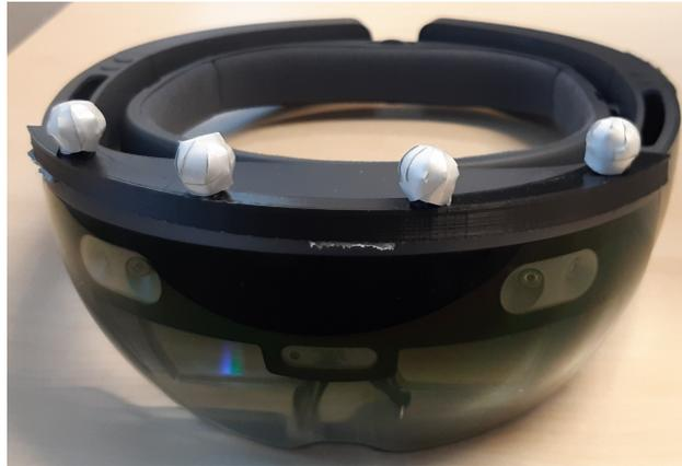
Figure 6: The HoloLens with the 3D printed bracket mounted on top of it. The markers were covered in retro reflective tape by hand such that they can be detected by the Optitrack system.
