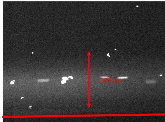
b. Chip 3, sample flow rate 2  $\mu\text{l}/\text{min}$ , sheath flow rate 40  $\mu\text{l}/\text{min}$ .
