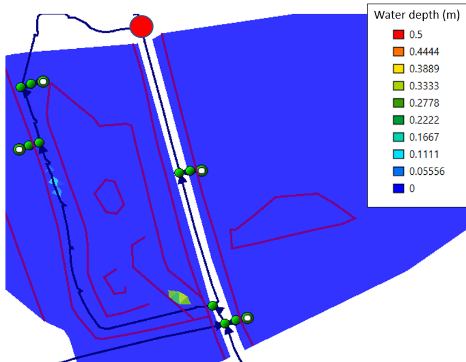
Figure 23 Simulated inundation at the Zandwetering grid during the peak flow (2020). As can be seen, only a few cells in 2D are active (all flow is through 1D). Water levels in the 1D network do not exceed the schematized bed level in 2D.
