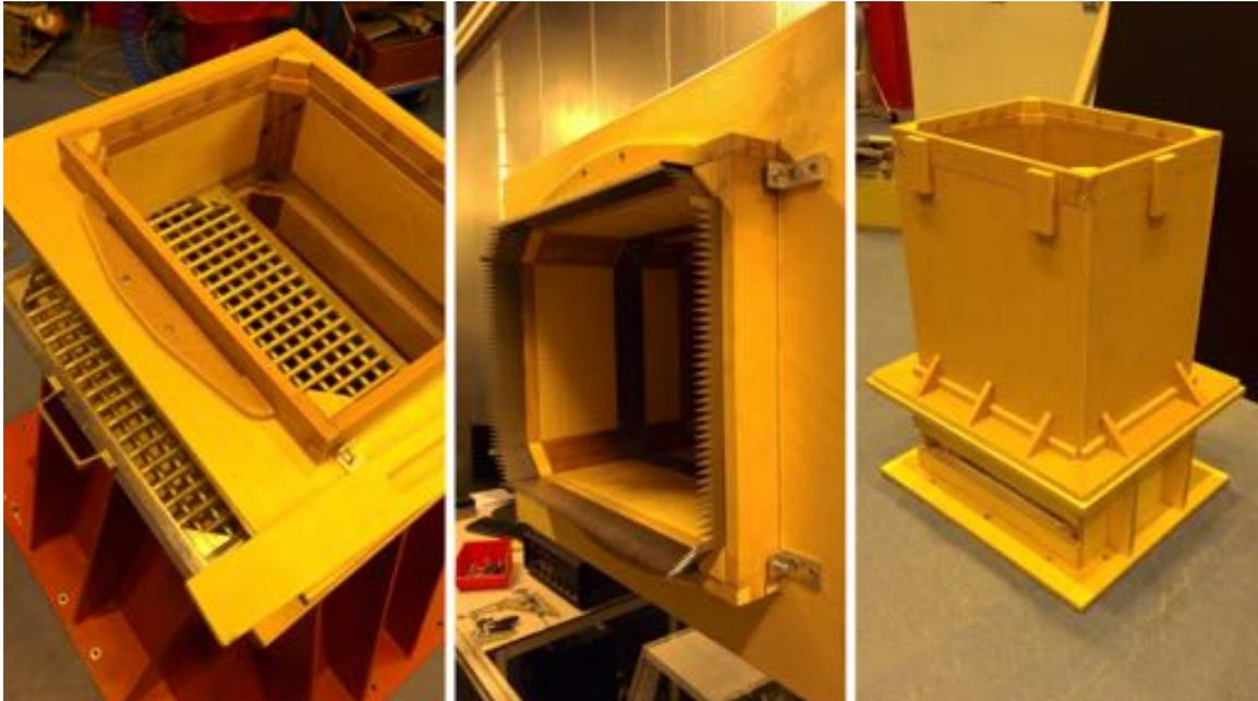
Figure C.3: Left: One of the turbulence grid being inserted into the slot in the wind tunnel section developed for interchangeable grids. Middle: Extension constructed to magnetically mount different serration profiles to the inlet nozzle. Right: The extension construction to extend the length of the inlet nozzle in order to direct grid noise down stream instead towards the microphones.
