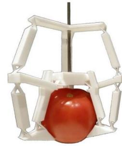
Figure 28: Linkage driven gripper [2]
