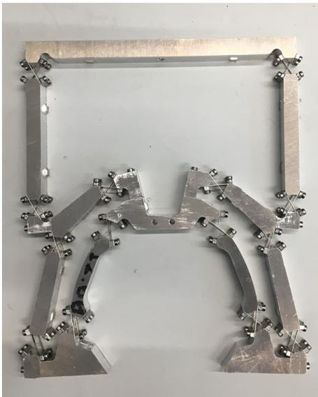
Figure 31: Metal gripper Aluminium and stainless steel hinges
