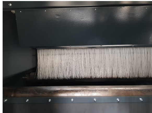
Figure 8 The brush, which is located on the inside of the brush/blow-off plant.
