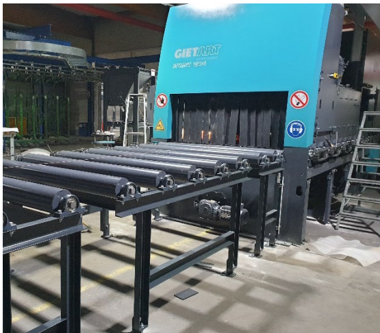
Figure 12: The roller conveyors located before the infeed of the shot blasting machine. The shot blasting machine is located at a customer.
