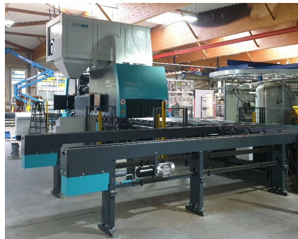
Figure 11: The cross conveyors, which transport the constructions sideways. The shot blasting machine is located at a customer.
