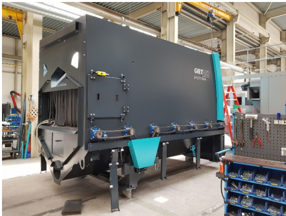
Figure 9: The brush/blow-off plant ready for expedition.
