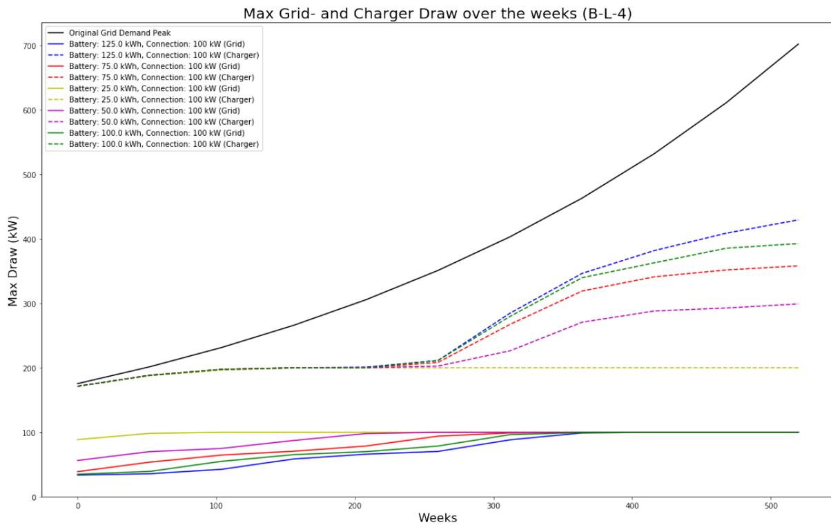
Figure B.15: Optimal Charger Draw Limit B-L-4
