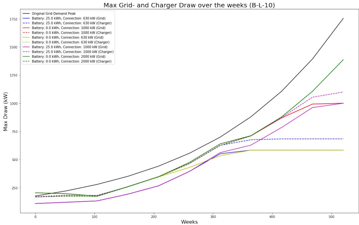
Figure B.17: Optimal Charger Draw Limit B-L-10
