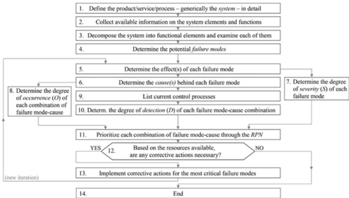
Figure 2.1: Flowchart showing stages of an FMEA [1]
