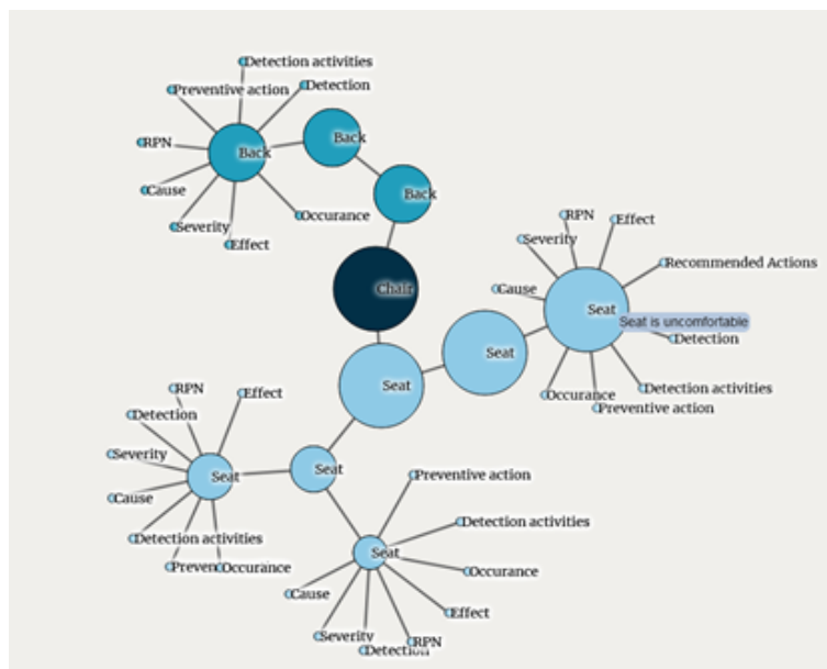
Figure 7.2: Prototype I, all nodes opened with all attributes of the Failure Modes accessible in node-form
