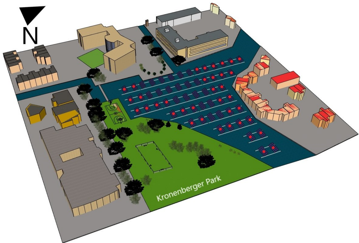
Figure 21: Digital 3-D model of the preliminary floating PV system and the location selected. The arrays that are subject to shading throughout the day and that would hinder the passage of boats are highlighted with a redpoint. They are not considered for the final sizing of the floating PV system.
