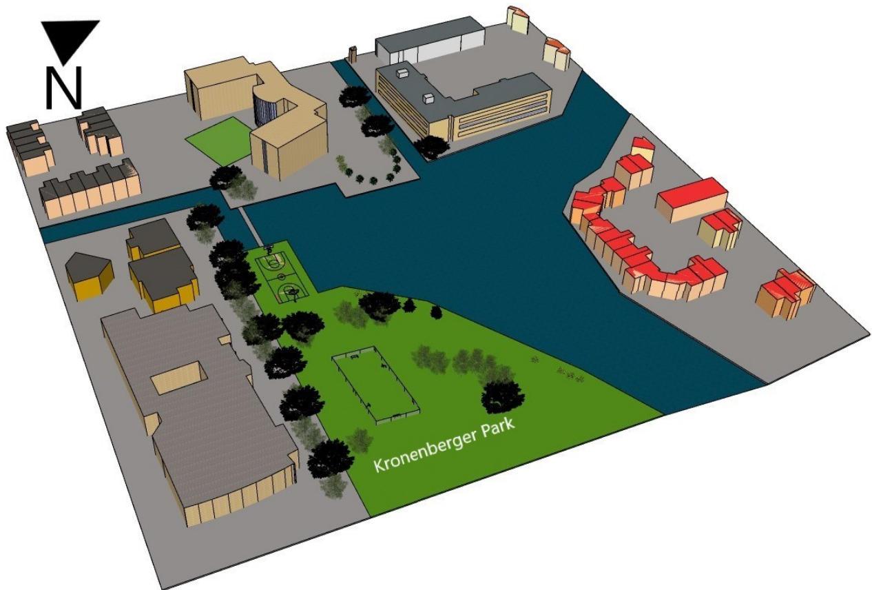
Figure 16: Digital 3-D model of the location in the Camminghaburen neighbourhood develop with SketchUp Pro 2021. This model is used to carry out an automatic shading analysis.
