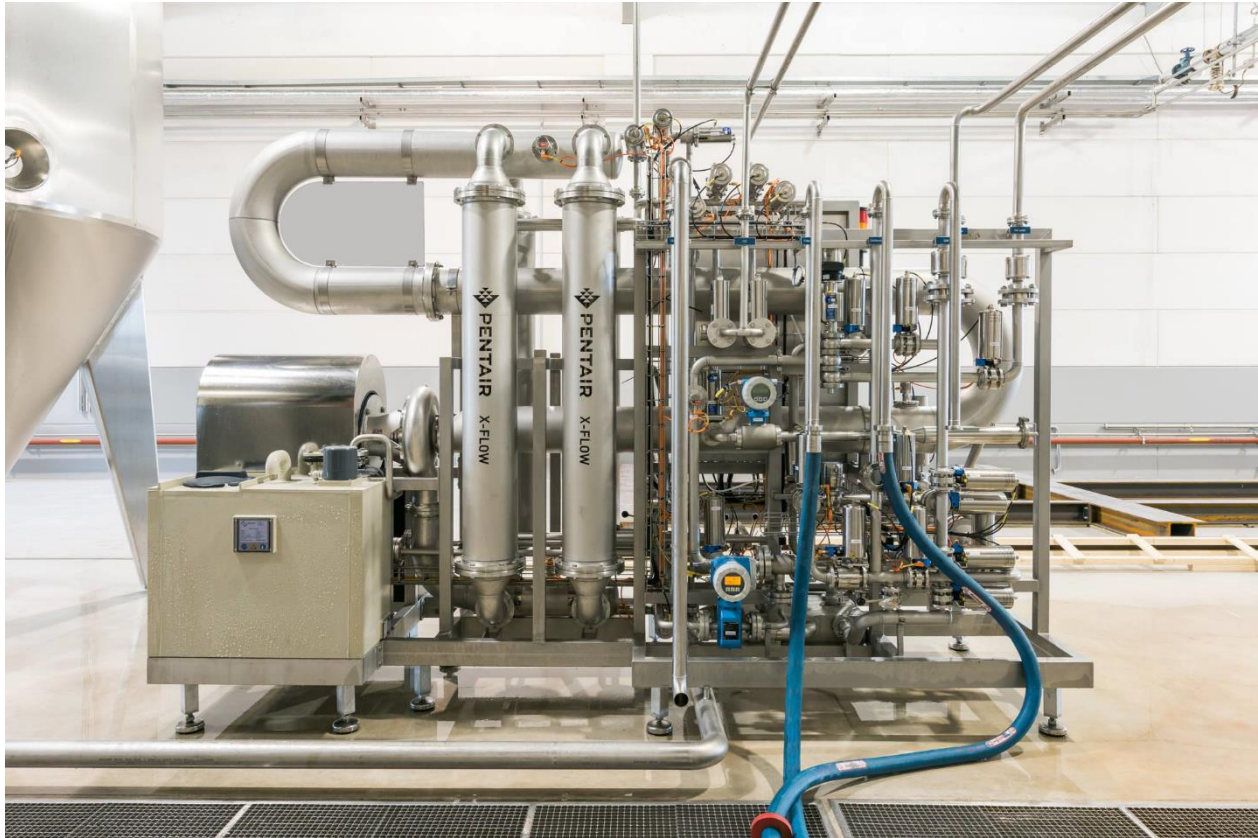
Figure 9: BMF+ Flux Compact S4 (source: Pentair)
