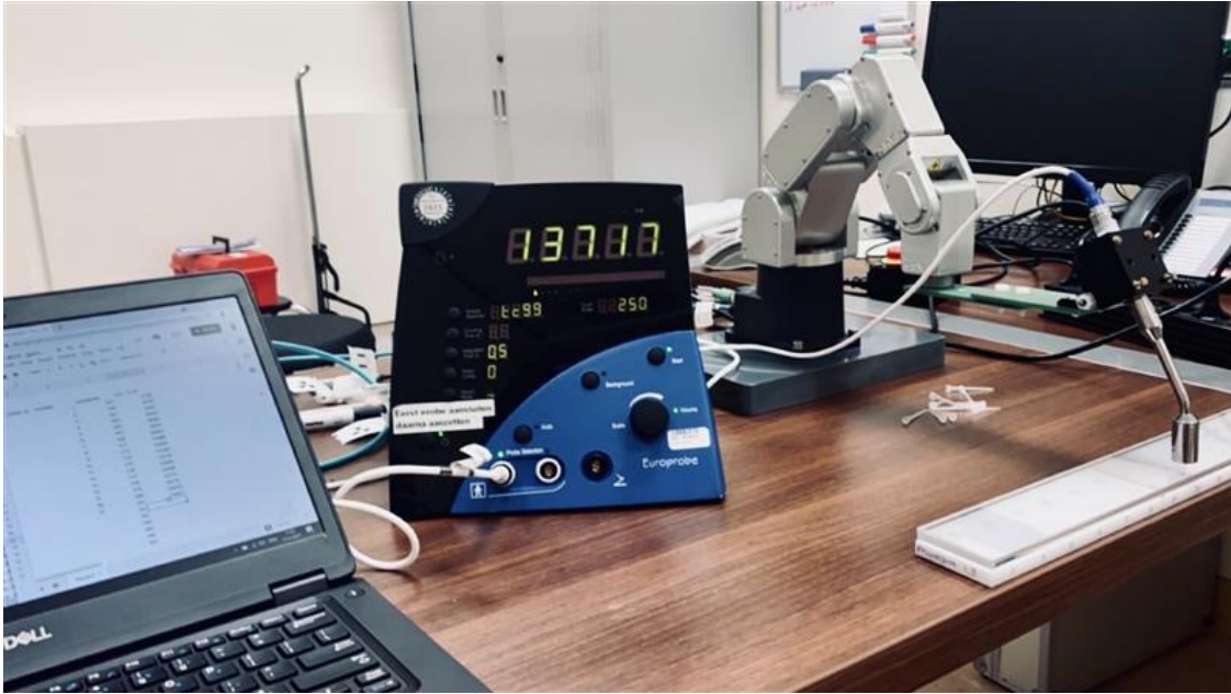
Figure 6: Experimental setup showing Europrobe3.2, Robotic arm, and phantom (with PMMA)
