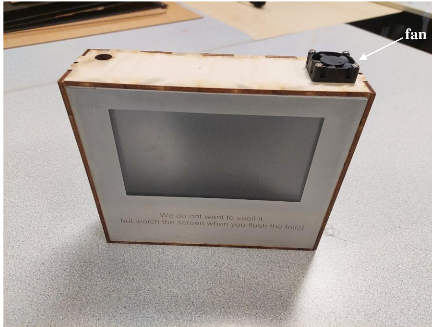
Figure 41: final case with screen and fan
