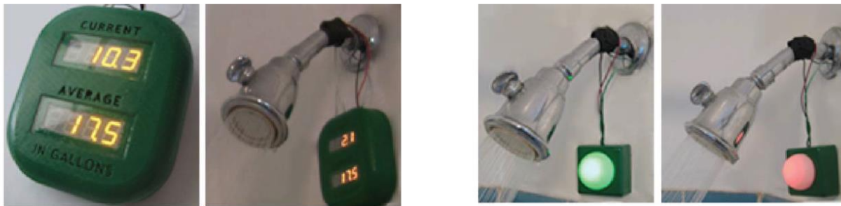
Figure 7: Intervention aimed at reducing water usage of a shower with metrics being used on the left and ambient feedback on the right [20].
