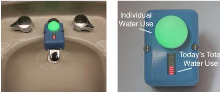
Figure 2: Water tap intervention that shows individual and total water use [20]
