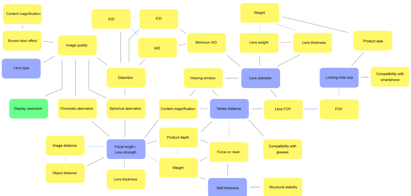
Figure 37: influence chart of the product, mapping how different variables affect each other
