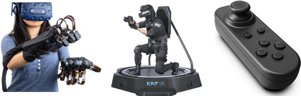
Figure 6-8: a haptic glove (left) a VR treadmill (middle) and a remote control (right)
