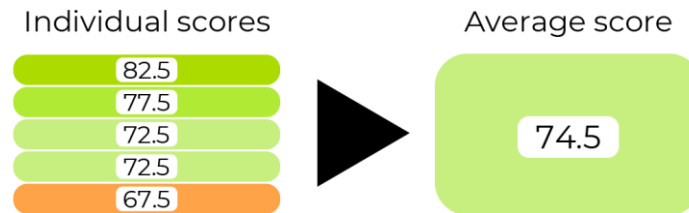
Figure 51: Representation of the System Usability Scale score for the 5 participants, leading to an average score
