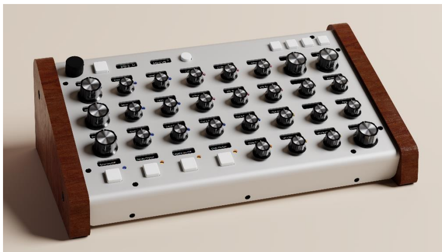
Figure 8: Modsy controller, with an exterior made of wood and aluminium [8]
