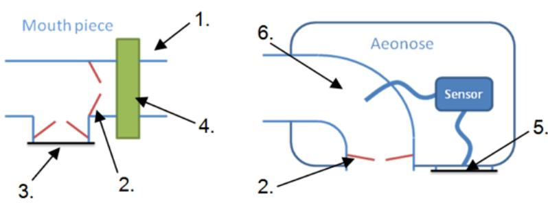
Figure 1: Electronic nose produced by the Enose company. Figure 2: Schematic drawing of the electronic nose. (1) disposable mouth piece, (2) one way valves, (3, 5) carbon filter, (4) HEPA filter, (6) sample chamber
