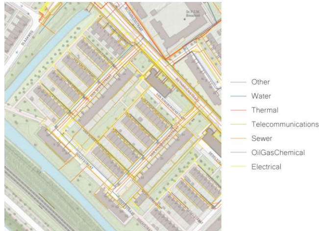
Figure 34: Underground utilities in case area 2
