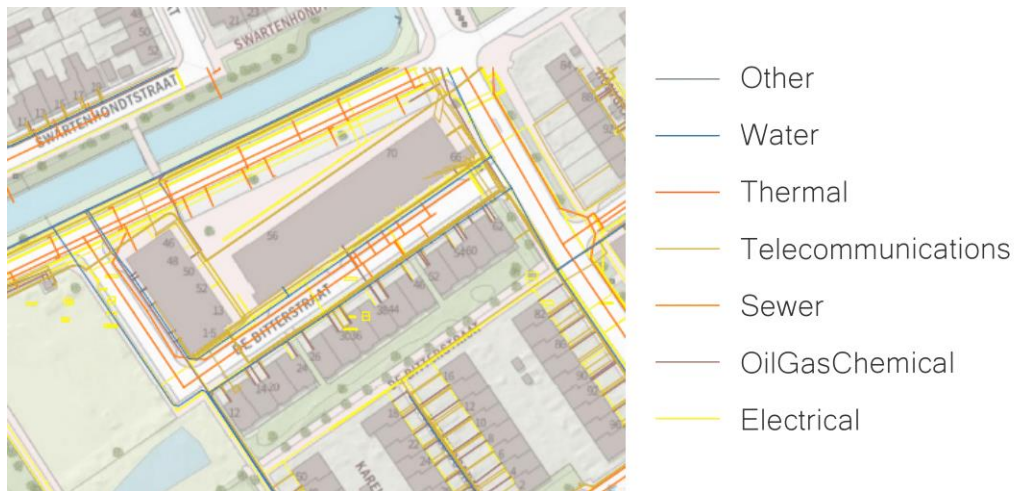
Figure 24: Underground utilities in the case area 1
