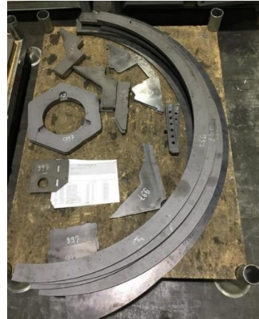
Figure 2-3: Cut parts out of the steel plates
