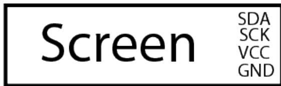
Figure 42: Pin layout of the screen,
