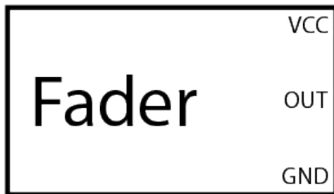
Figure 40: Pin layout of the fader
