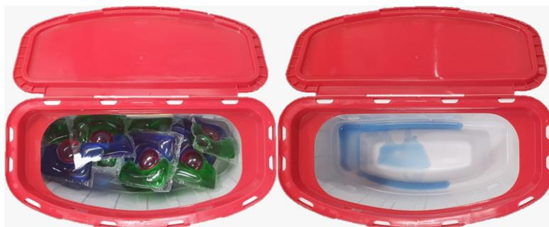
FIGURE 1.1: Example of Leakage inside Detergent Pod Container
