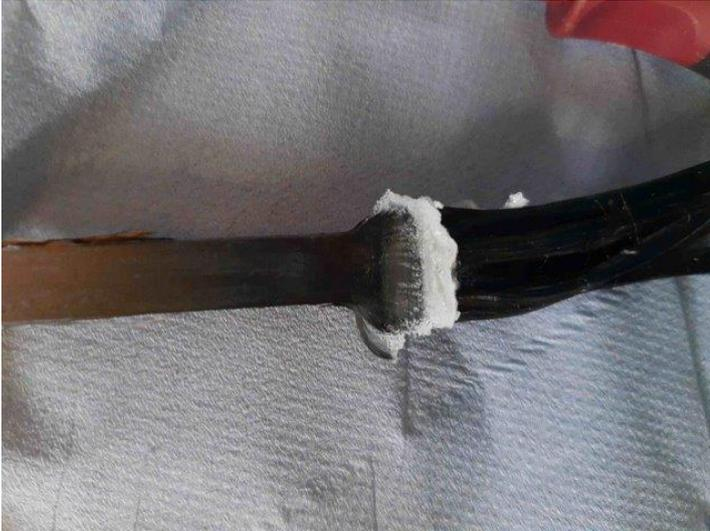
Figure 23: Material stuck in the die entrance
