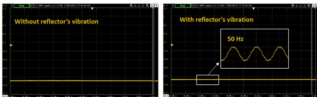
**Figure 5.6:** Optical testing result with the  $850nm$  wavelength laser diode and vibrated reflector.
