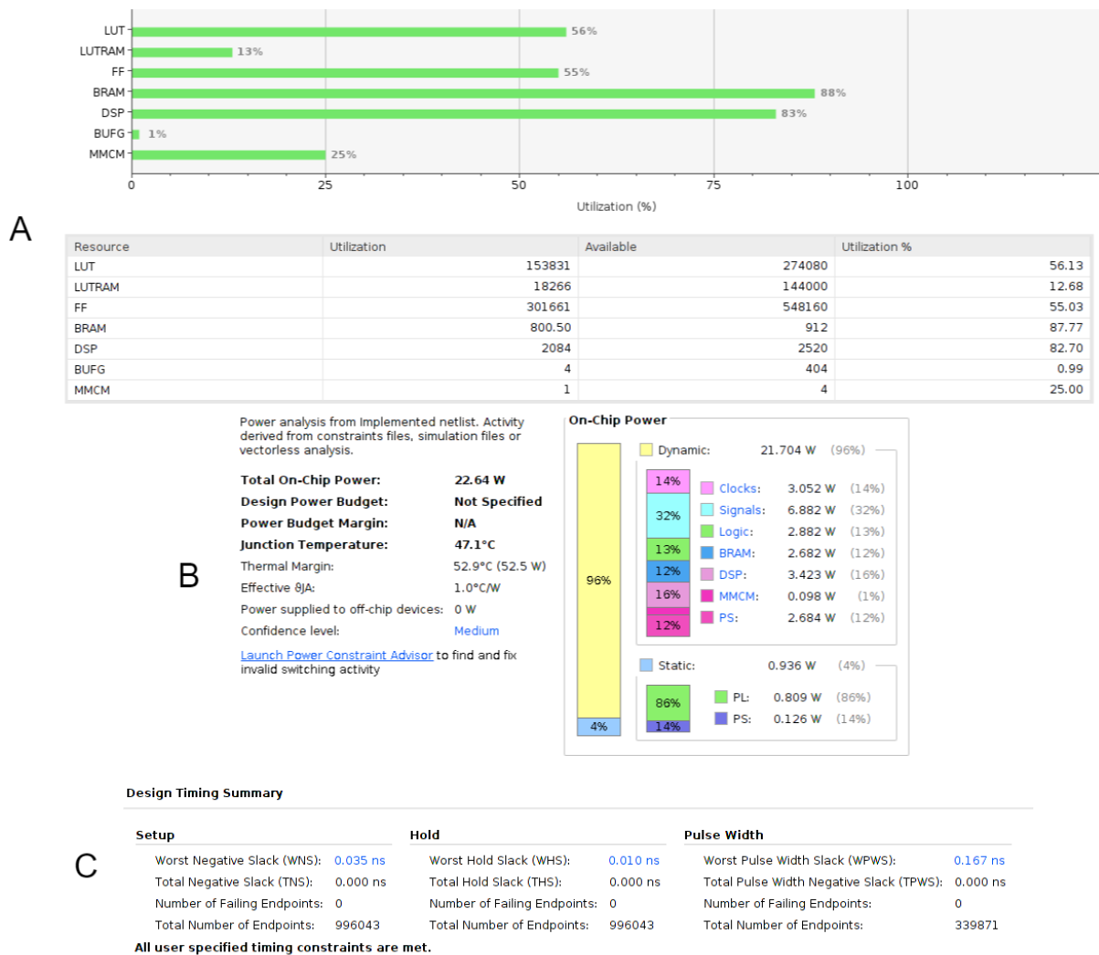
Figure 6.11: Vitis Analyzer DPUCZDX8G on a ZCU102, 3 DPU core B4096, running on 150MHz, synthesized, A shows resource usage, B shows timing summary, and C shows power summary
