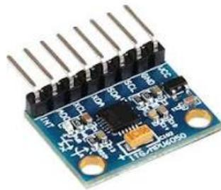
Figure 3.2: 6-axis IMU sensor (MPU6050)
