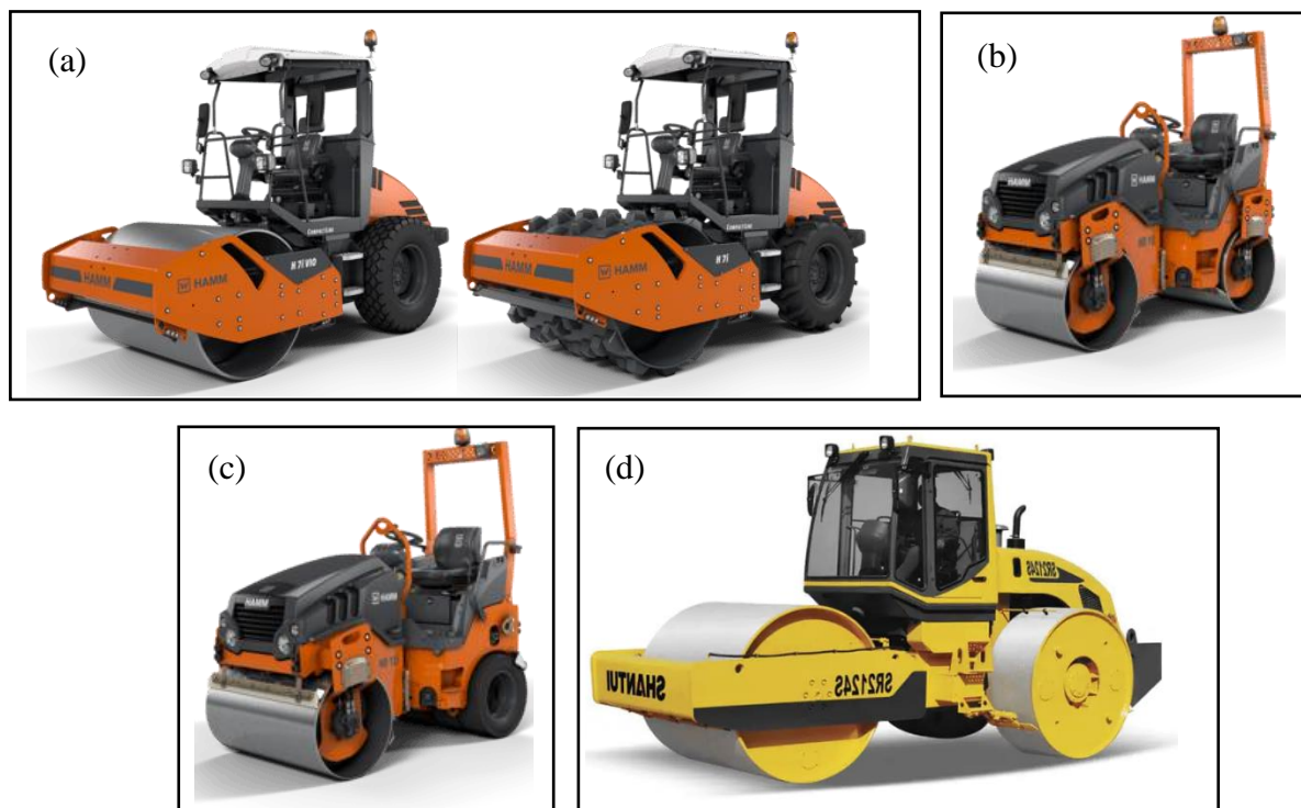
Figure 10: (a) compactors; (b) tandem rollers; (c) rubbed rollers; (d) static three-wheeled rollers. Adapted from (ArchiExpo, n.d.; Wirtgen Group, n.d.)
