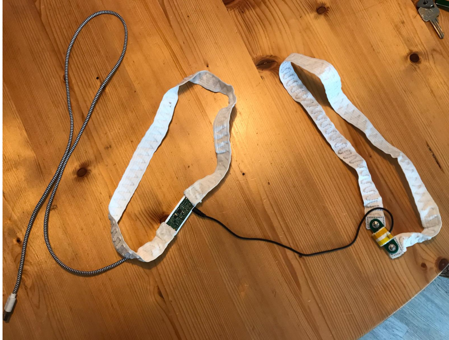
Figure 18: Respiration sensor. The left band is to measure breath for the abdomen and the right one for the chest
