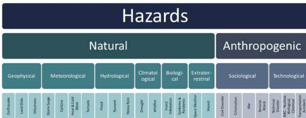
Figure 1 : Types of Hazards
