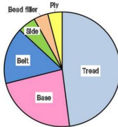
Figure 10: Energy loss in each part of the tire (Akutagawa, 2017)
