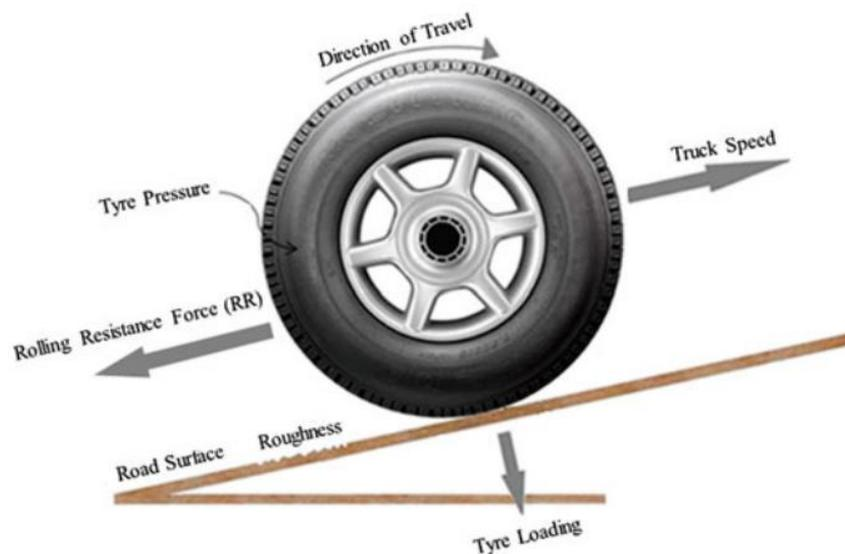
Figure 1: Rolling resistance acting on a tire (Soofastaei & Karimpour, 2008)
