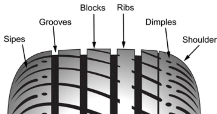
Figure 2: Tire tread design with its main components (Companies, 2015)
