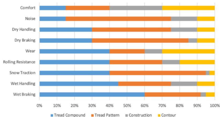
Figure 9: Tire components contribution to each phenomenon in % (Niknam, 2021).
