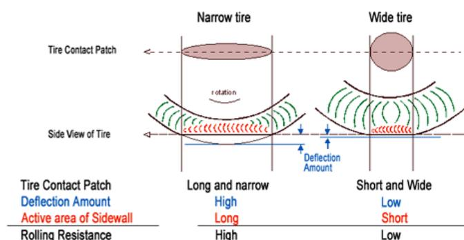
Figure 3: Tire size effect on rolling resistance (Artisanales, 2006)
