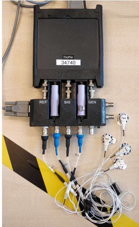
**Figure 3.1:** The TiePie oscilloscope, top black box, connected with three coax connections to the custom PCB (bottom black box). Two measurement connections and one connects to the waveform generator. The used coax cables connect the electrodes with the four PCB outputs,  $H_{\text{cur,I}}$ ,  $H_{\text{pot}}$ ,  $L_{\text{pot}}$  and  $L_{\text{cur}}$ .
