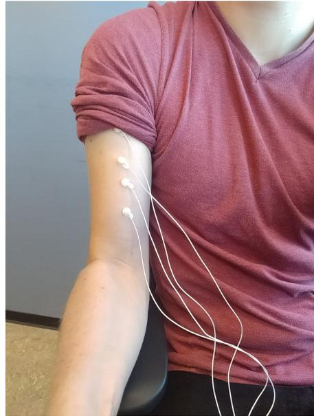
**Figure 3.2:** The electrodes as they are placed on the arm. The smaller electrodes are used in this picture. The electrodes are connected to the PCB as follows, from high to low:  $H_{\text{cur},I}$ ,  $H_{\text{pot}}$ ,  $L_{\text{pot}}$  and  $L_{\text{cur}}$ .
