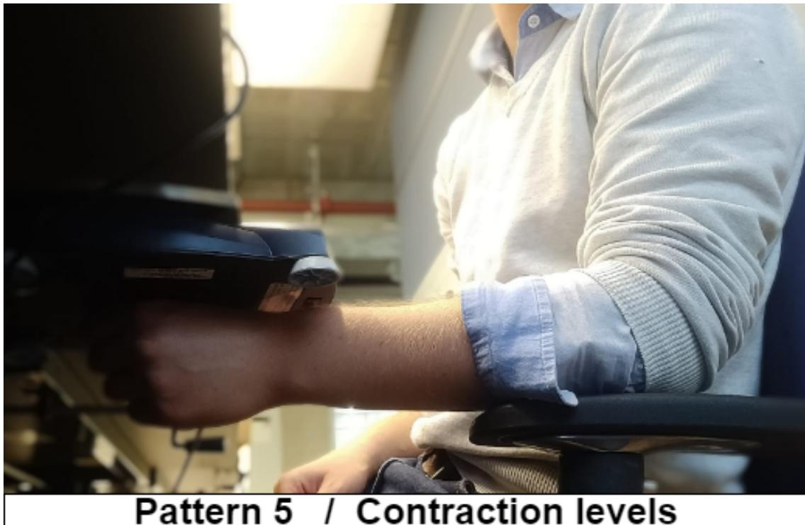
**Figure 3.13:** Movement pattern 5. The weighting scale is placed on top of the hand beneath a table top.
