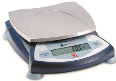
**Figure 3.12:** The used weighting scale, Ohaus Scout Pro 6001. The maximum weight is 6 kg with a resolution of 0.1 g.
