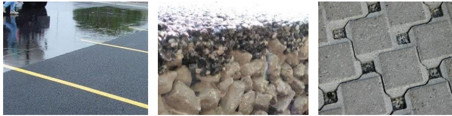
Figure 30 - Example of (f.l.t.r.) permeable asphalt (Mrugacz, 2017), permeable concrete (New Dawn, 2015), and permeable interlocking pavers (Sustainable Technologies, 2021)
