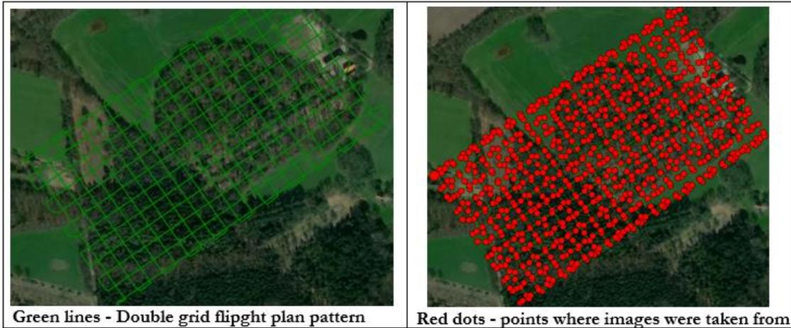
Figure 3: UAV flight plan.
